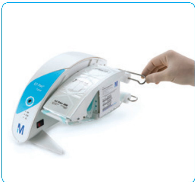
Step 3 Attach upper and lower packaging layers to the spools.
