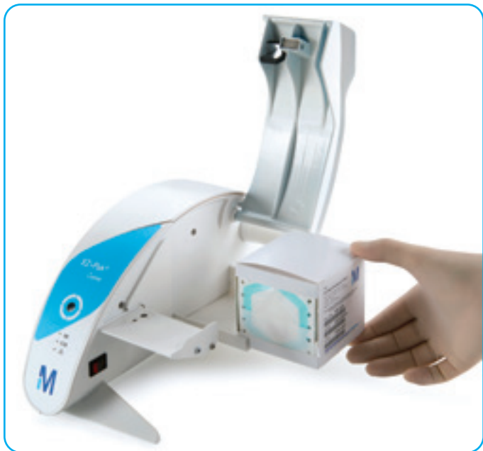
Step 1 Open cover and insert the cartridge.
